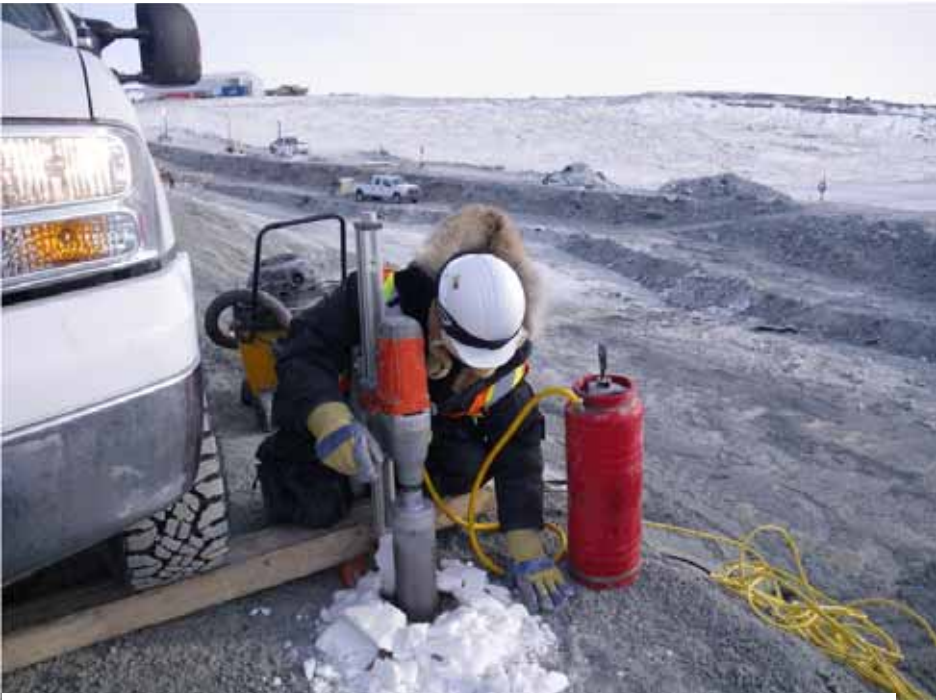
Photo 3: Collecting a drilled core sample. Coring! Coring!
